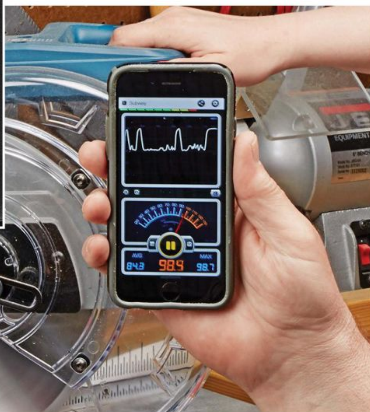
▲ The smartphone app from Decibel X Pro lets you take instant readings and record the noise levels in your shop. The app comes with directions for use (inset photo).
