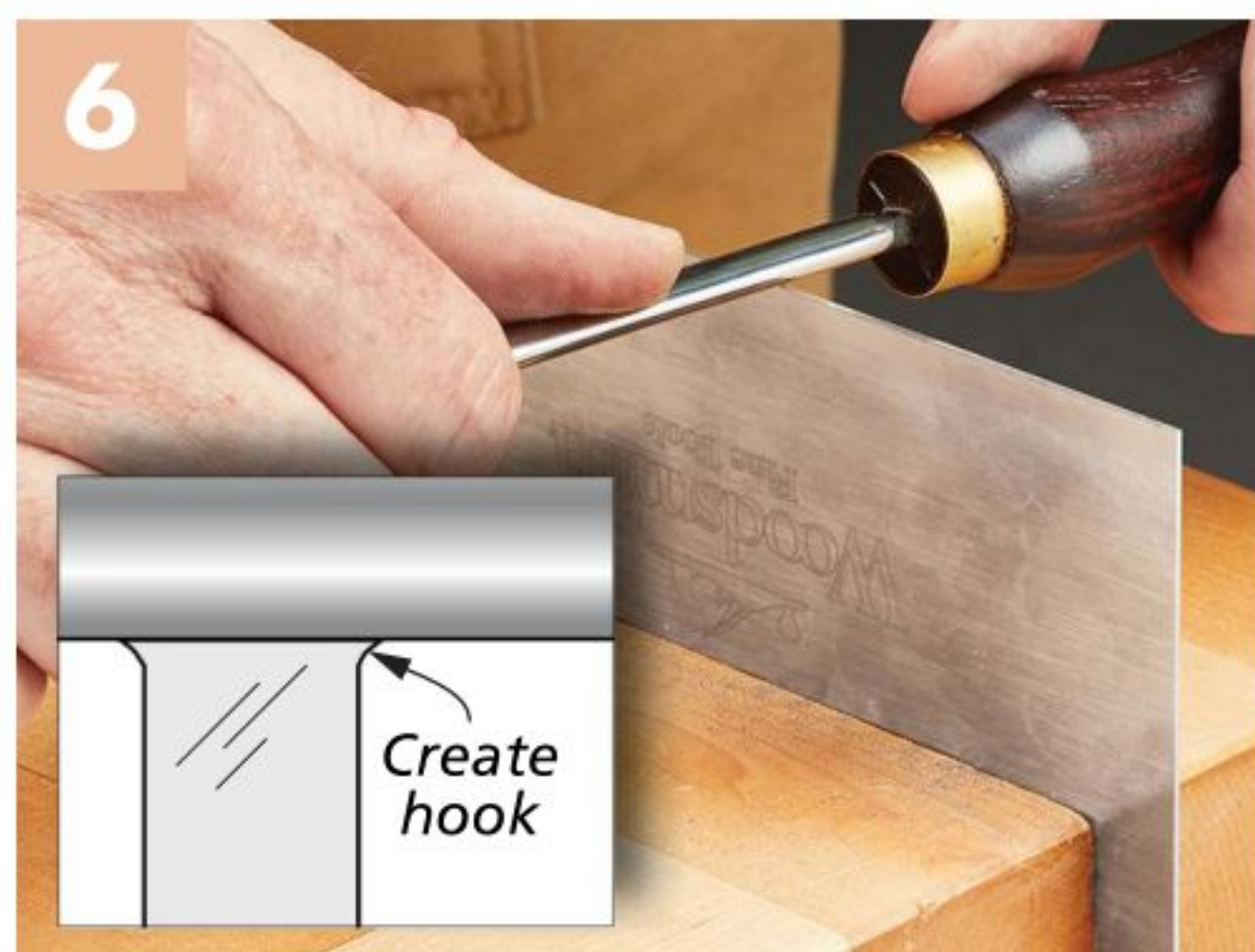
▲ Pressing the burnisher against the edge begins to form the hook, as shown in the inset drawing.
