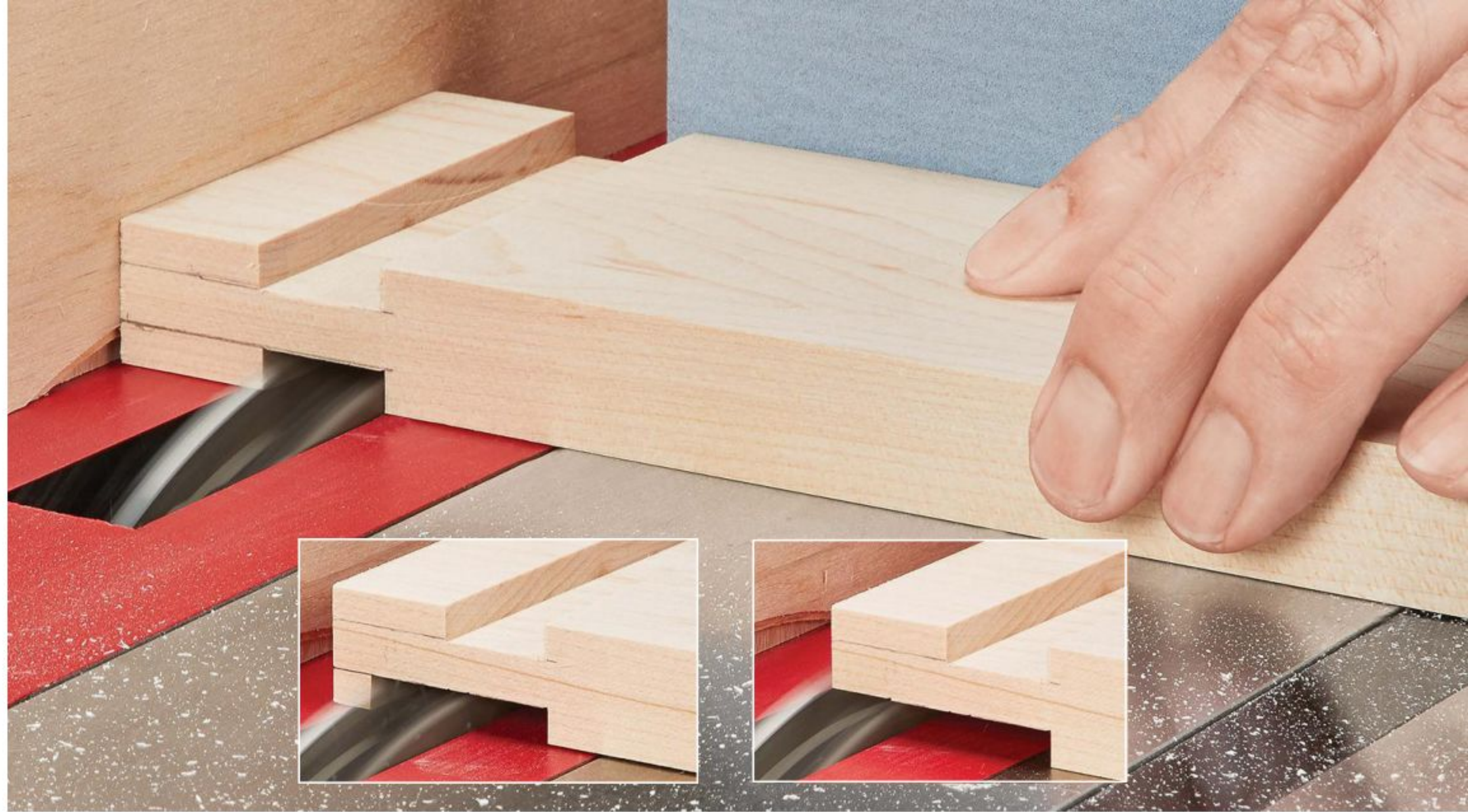
▲ When using a dado blade, use an auxiliary rip fence as a stop and form the tenon shoulders on both faces of the workpiece. Then, move the workpiece away from the fence and make continual passes to remove the remaining waste (inset photos).
