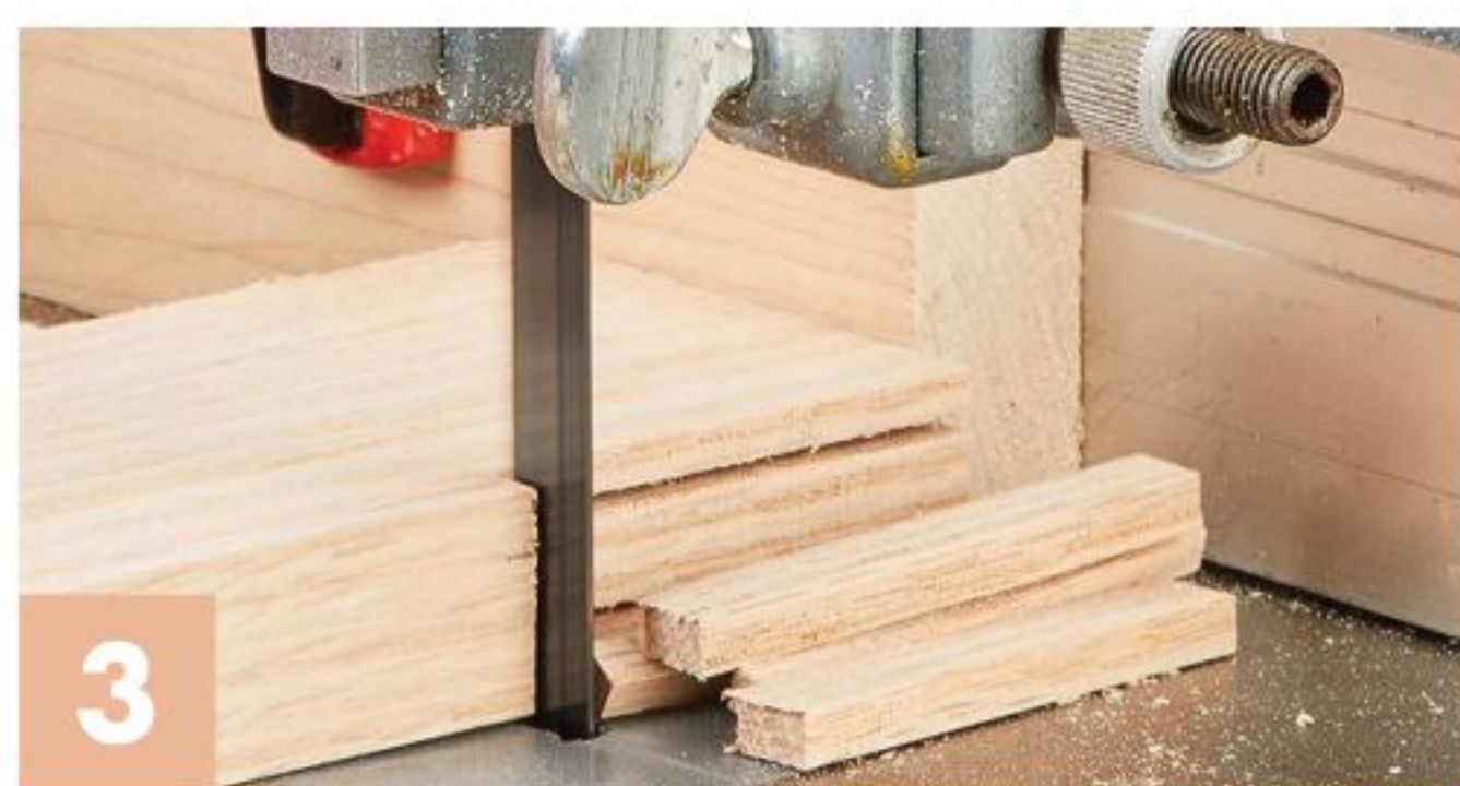
▲ Lay the piece flat and make the narrow cheek cuts (top). Then make the shoulder cut to remove the edge waste (bottom).
