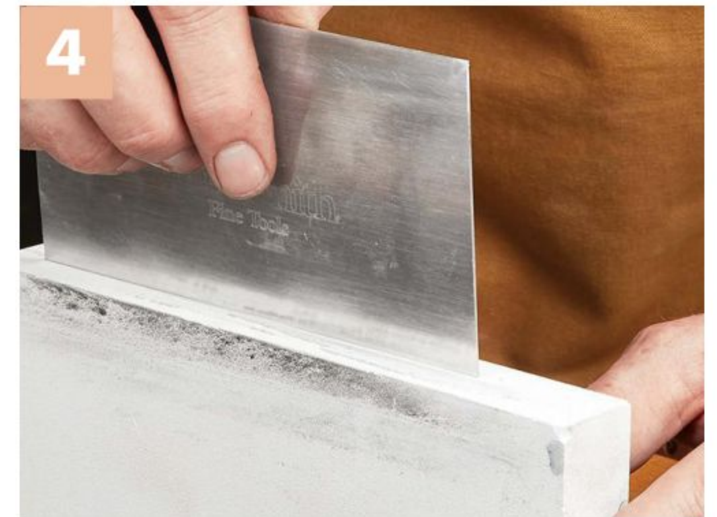
▲ Polish the edge, as well. Here it's best to use the edge of the stone to avoid grooving the face of the stone.
