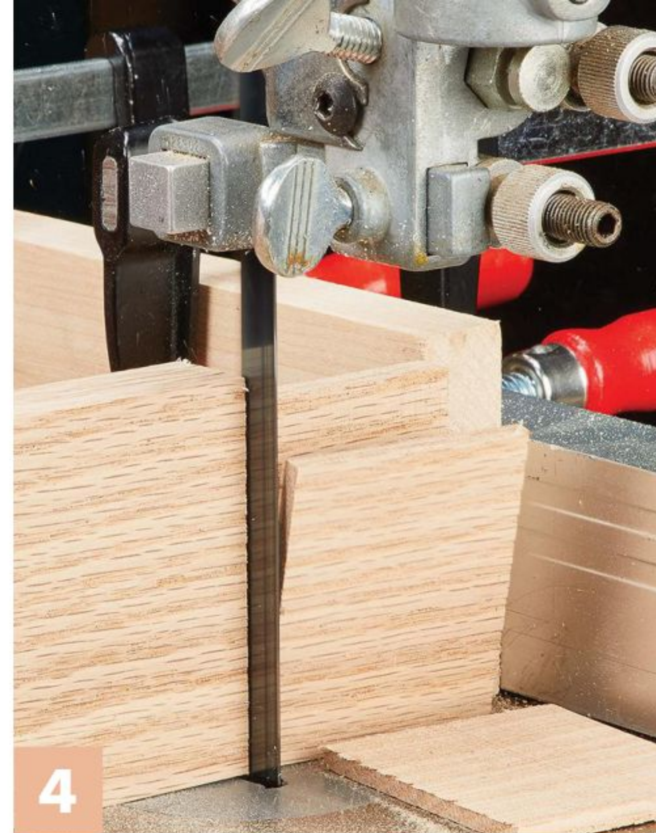
▲ Stand the workpiece on edge again and, using a miter gauge, make the shoulder cut on the wide face of the workpiece.
