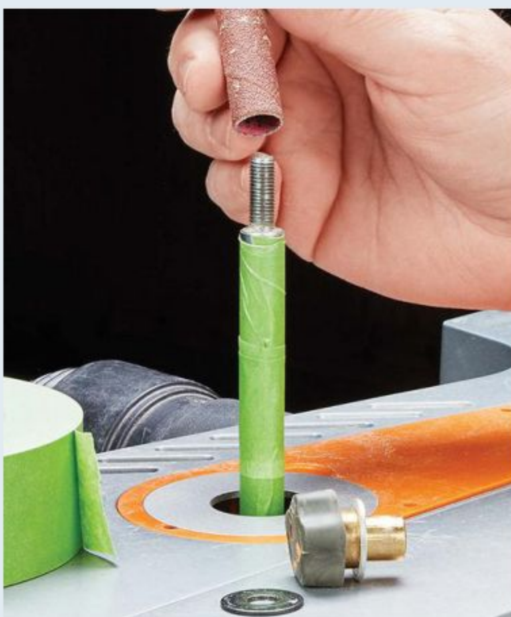
Knobless Sander. Riley Onofrio of Saint Paul, MN, needed to sand a tall workpiece on his spindle sander but the retaining knob at the top hit the workpiece as it oscillated. To fix the problem, Riley used a few layers of painter's tape on the shaft. The friction holds the sleeve in place without the knob.
