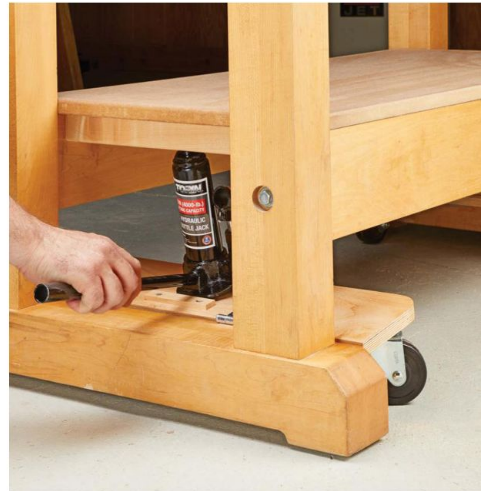
▲ Pumping up the jack raises the foot off the floor. Lowering the jack drops the bench back onto the foot.
