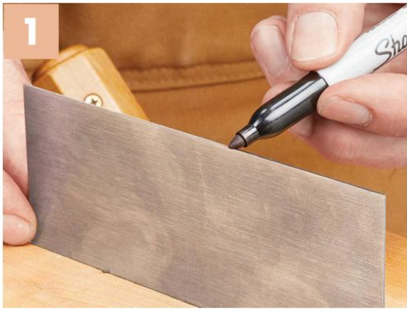
▲ Running a marker along the edge helps provide a good gauge of progress as you reshape and straighten the edge.
