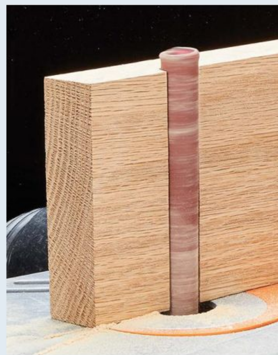
Knobless Sander. Riley Onofrio of Saint Paul, MN, needed to sand a tall workpiece on his spindle sander but the retaining knob at the top hit the workpiece as it oscillated. To fix the problem, Riley used a few layers of painter's tape on the shaft. The friction holds the sleeve in place without the knob.
