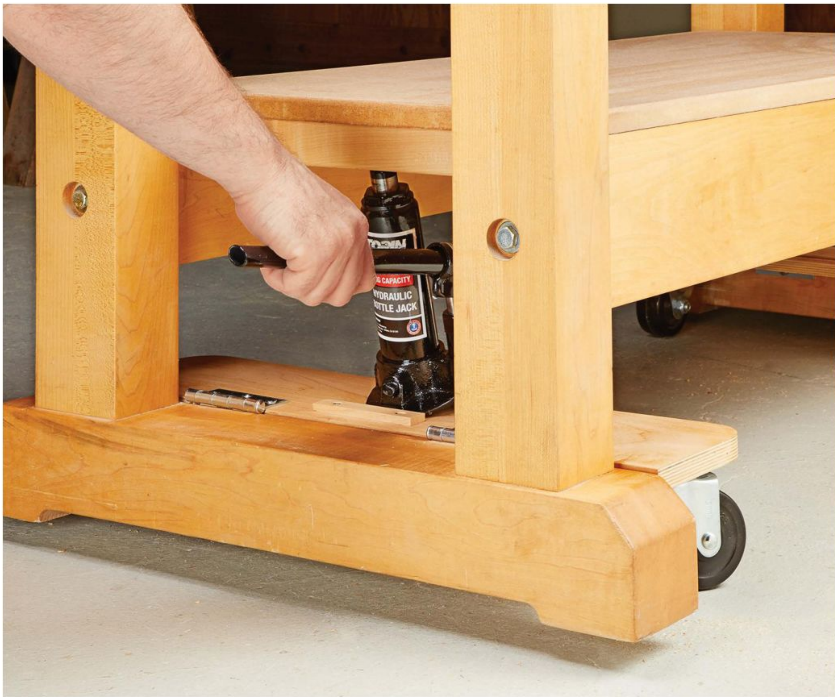
▲ Pumping up the jack raises the foot off the floor. Lowering the jack drops the bench back onto the foot.
