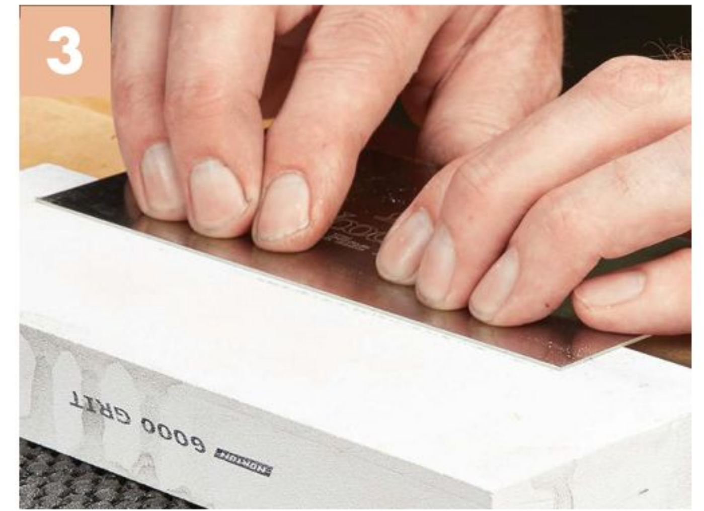
▲ Polish each face and edge of the scraper, working your way up from the 1000-grit stone to the 6000-grit.
