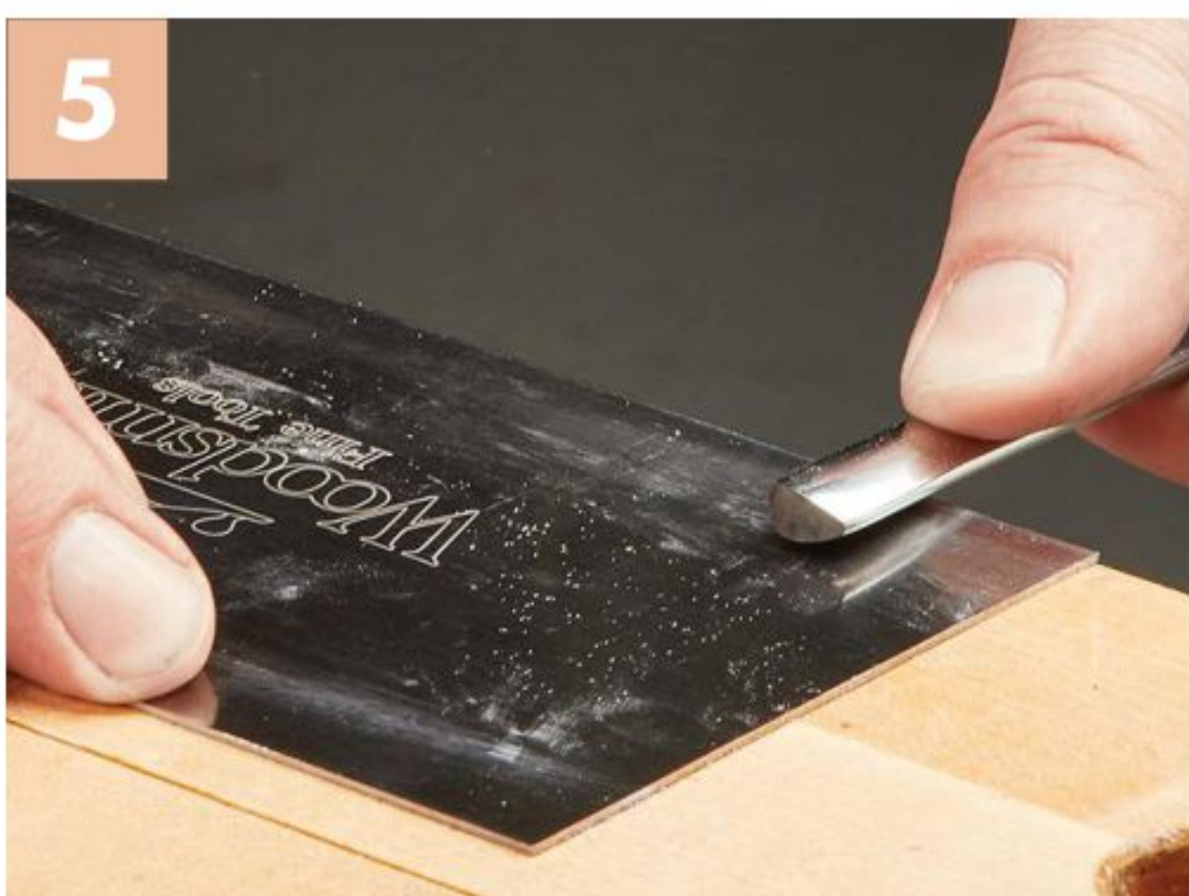
▲ With the scraper flat on the bench, press the burnisher firmly down as you push it along the surface.
