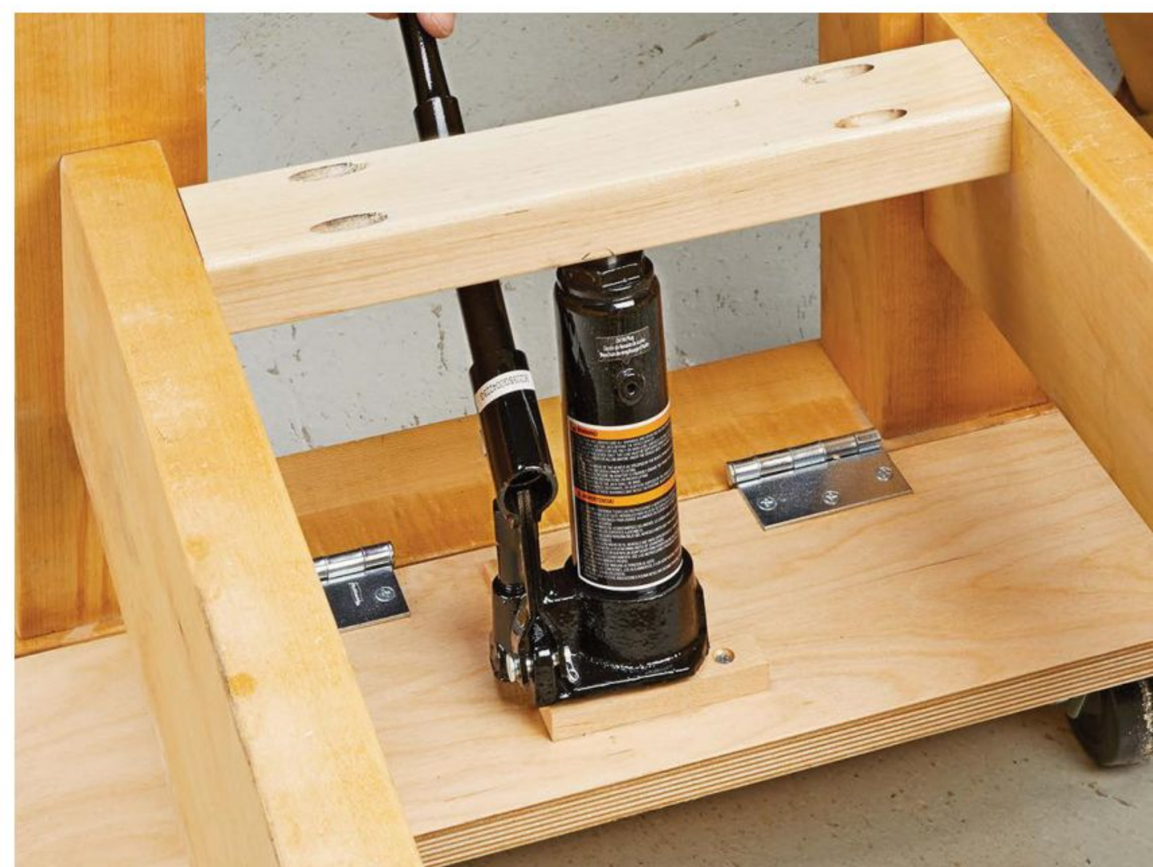
▲ The jack rests on a hinged plate with cleats to hold the jack in place. When pumping up the jack, it presses against the lower shelf support and lowers the plate and wheels, raising the bench.
