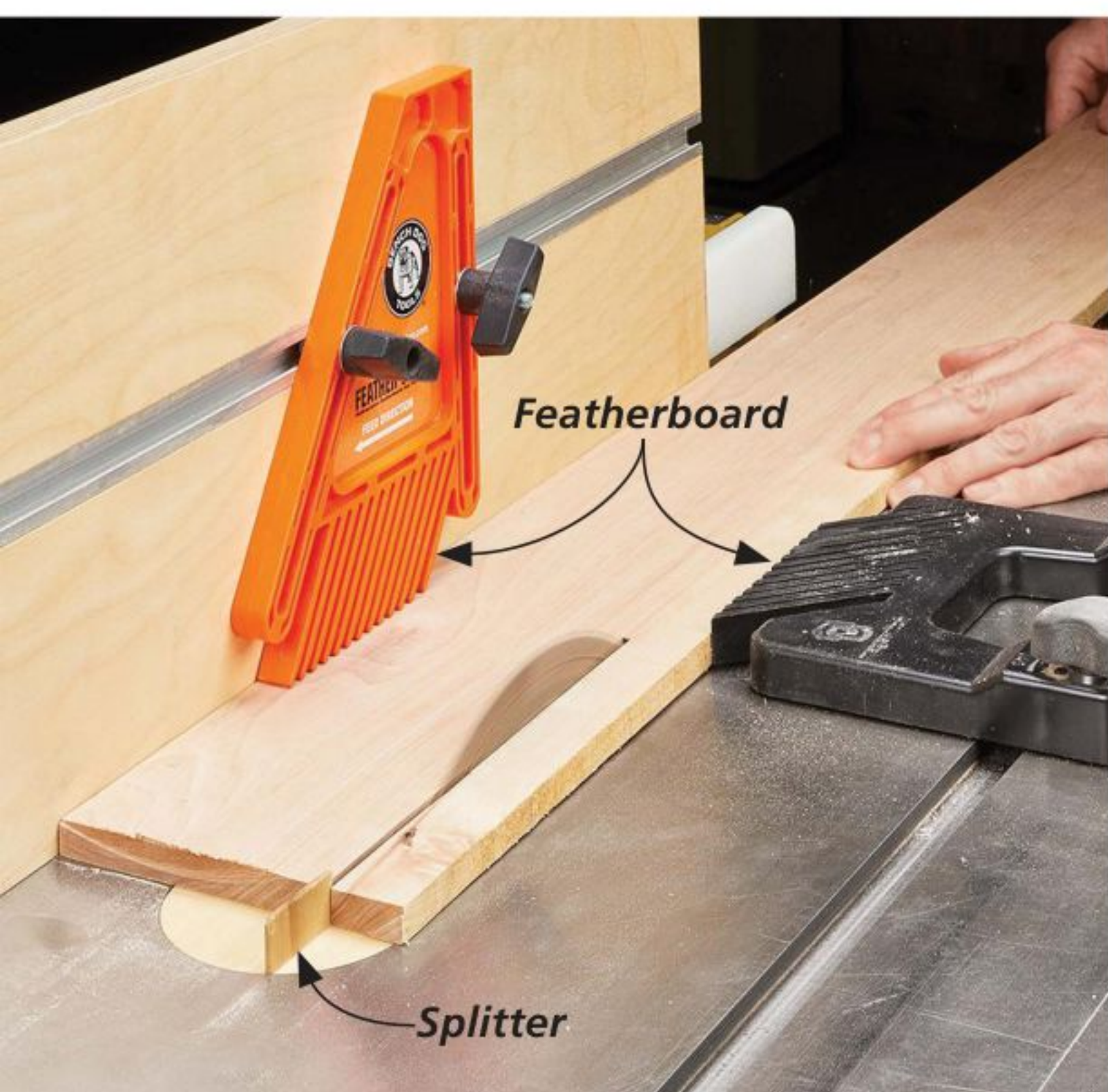
▲ Featherboards (above), hold-downs (main photo) and a splitter or riving knife (inset) are essential for safe rip cuts.
